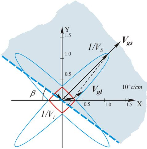
Fig. 1. Acoustic reflection from the boundary between a paratellurite crystal and vacuum involves a transformation of modes, which can be illustrated by a scheme that depicts the process.
