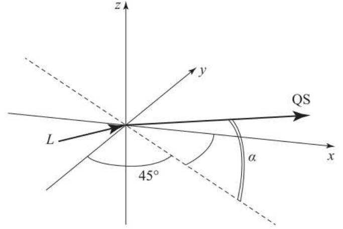
Fig. 2. The conversion of a longitudinal acoustic wave L, propagating outside the principal plane, into a slow quasi-transverse QSS wave.
