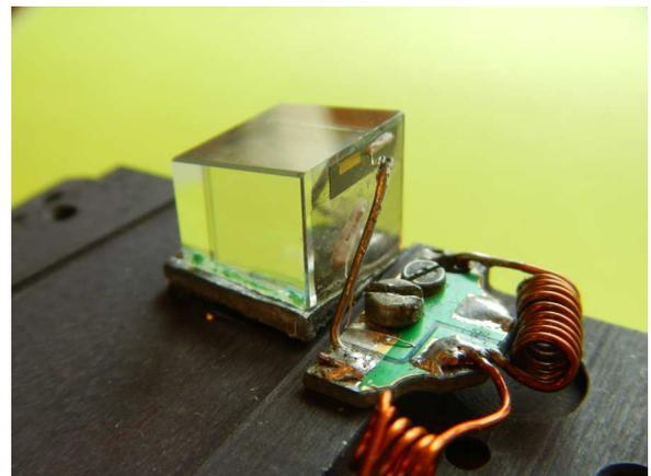
Fig. 4. An acousto-optic device that utilizes a paratellurite crystal as its core component.
