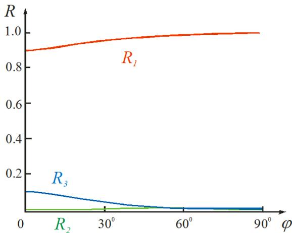
Fig. 3. The energy reflection coefficients in the crystal plane depending on the angle  $\alpha$ .
