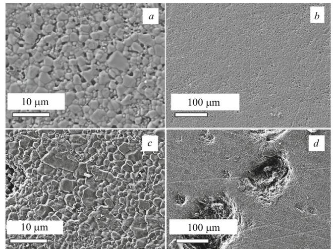
**Fig. 4.** Photomicrographs of thin sections of ceramic obtained from OCP powder: *a, b*) OCP-450; *c, d*) OCP-600; firing temperature 1100°C, soaking time 3 h.
