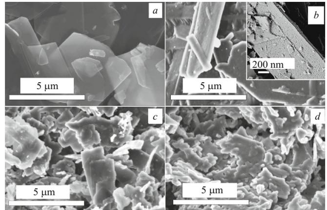
**Fig. 1.** Photomicrographs of OCP and its products of heat-treatment: single-phase OCP was synthesized in an acetate buffer solution at 60°C and pH = 5.75; a) OCP powder without heat-treatment; b) OCP powder heat-treated at 450°C (OCP-450); c) at 600°C (OCP-600); d) at 700°C (OCP-700).
