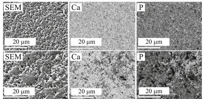
**Fig. 6.** Photomicrograph of a thin section of ceramic made from OCP-450 (top) and a thin section of ceramic made from TCP/ CPP (bottom) and maps of the calcium and phosphorus distributions in them: in the maps of the phosphorus distribution the light-colored sections correspond to calcium pyrophosphate.
