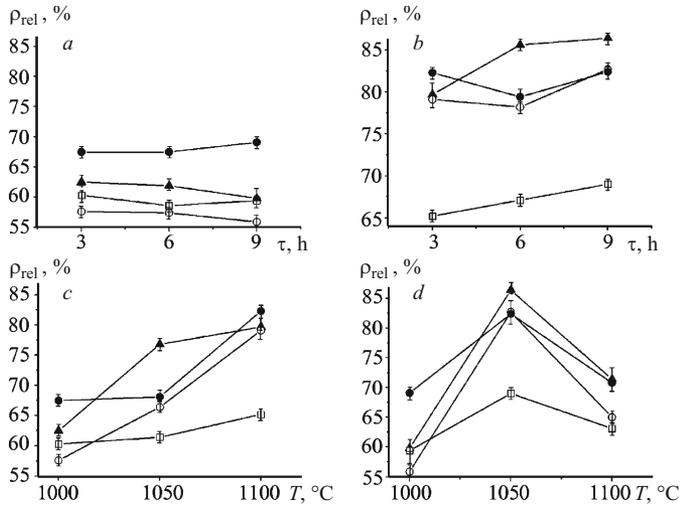
**Fig. 2.** Relative density of ceramic versus heat treatment conditions: *a, b*) firing temperature 1000 and 1100°C, respectively, with different isothermal soaking times; *c, d*) isothermal soaking for 3 and 9 h, respectively, at different firing temperature; □) TCP/CPP; ▲) OCP-450; ○) OCP-600; ●) OCP-700.
