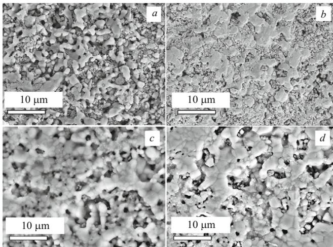
**Fig. 3.** Photomicrographs of thin sections of ceramic obtained from a mechanical mixture of powders TCP/CPP at firing temperature: *a*) 1000°C, 3 h; *b*) 1000°C, 9 h; *c*) 1100°C, 3 h; *d*) 1100°C, 9 h.
