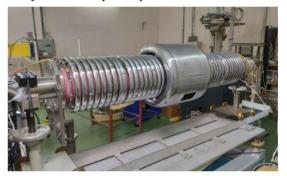
Figure 3: Accelerator tube assembly for Tandem v.2.
