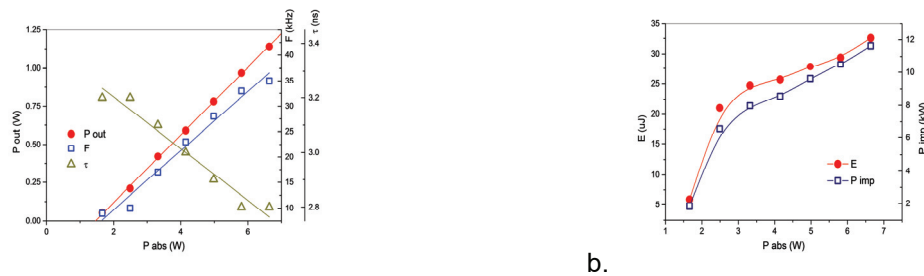
Fig.4 a. The average output power, the pulse width and the pulse-repetition rate and b. The pulse energy and the peak power of var-cut ( \theta=25^\circ , \varphi=0 ) \text{Nd}^{3+}:\text{GdVO}_4 passively Q-switched lasers vs absorbed pump power.
