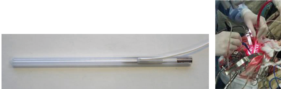
Fig.3. Sapphire multichannel probe for neurosurgery. Surgical operation on brain tumor removal using the sapphire probe for neurosurgery
