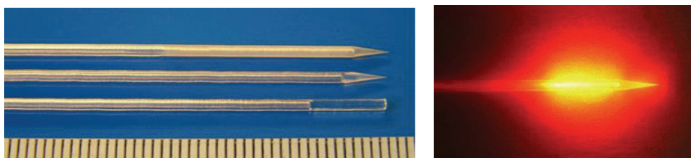
Fig.2. At the left: sapphire needle capillaries (external diameter of 1.2 mm, internal diameter of 0.5 mm): (a) as grown closed capillary; (b) capillary with a point formed by mechanical operation of the butt; (c) capillary with a point and diffuser formed by mechanical operation. At the right: sapphire needle combined with quartz fiber (the geometry of light field). The geometry of light field in sapphire needle (OD 1.2 mm, ID 0.5 mm) combined with quartz fiber.
