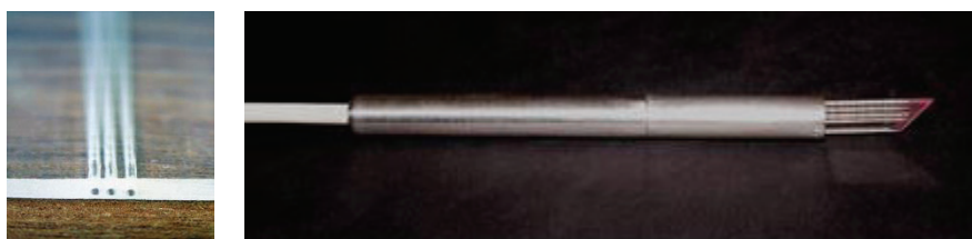
Fig.1. Sapphire ribbon with three capillary channels of 0.5 mm in diameter (at the left). Sapphire scalpel for diagnostic and coagulation on incised tissue during a surgical operation (at the right).
