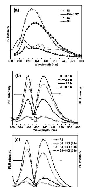
**Figure 6.** (a) PL spectra of samples S1, S2 (dried powder), S3 (PL intensity of the latter being multiplied 10 times), and S4. (b) Time evolution of PL and PLE spectra of heated mixture of S2 and OA from 0.5 to 3.5 h. (c) Time evolution of PL and PLE spectra of heated mixture of S1 and HCl over time range from 1 to 8 h.
