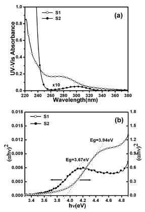
**Figure 5.** (a) UV—vis absorption spectra of S1 (with OA) and S2 (without OA); the absorption intensity of S2 is multiplied 10 times. (b)  $(\alpha h\nu)^2$  versus  $h\nu$  plot for determining absorption onset of S1 and S2.
