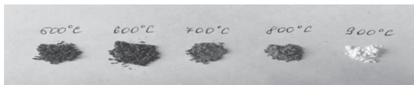
Figure 1. \text{Ca}_2\text{P}_2\text{O}_7 powders, synthesized from \text{Ca}(\text{CH}_3\text{COO})_2 and (\text{NH}_4)_4\text{P}_2\text{O}_7 , after heat treatment at different temperatures.
