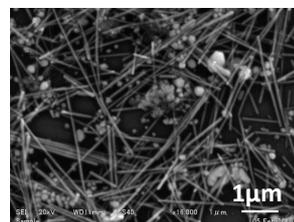
Fig. 2 SEM image of AgNWs grown and crosslinked to the surface-treated Si wafer.
