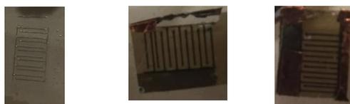
Fig. 1: Pictures showing different geometries of electrodes made of GO dried on PET.
