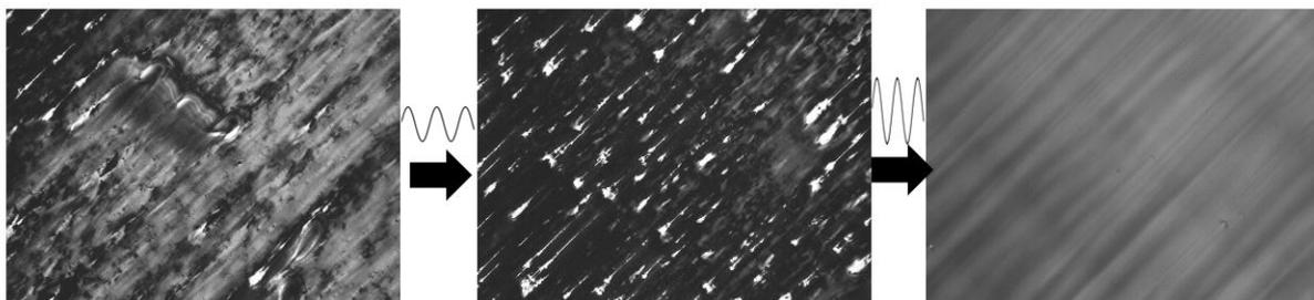
*Fig. 1: From the left to right: Meniscus-guided coating of a D-A polymer with several types of non-uniformities; coating of a film with vibration and low acceleration; coating of a film with vibration and high acceleration.*
