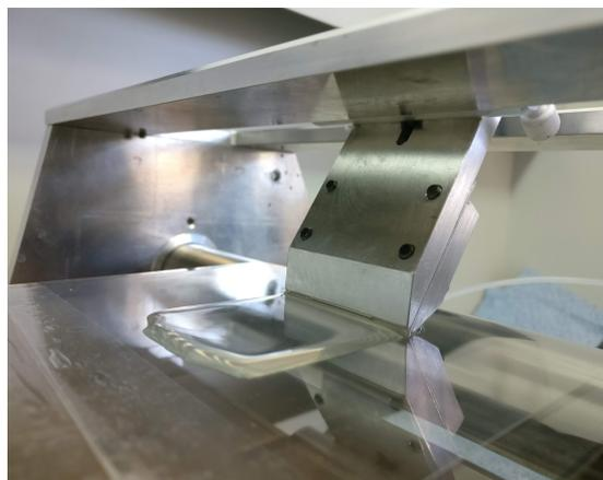
Figure 1: a photograph of the slot dye coating system used to prepare large area (25 x 5 cm<sup>2</sup>) chitosan-based IPN membranes
