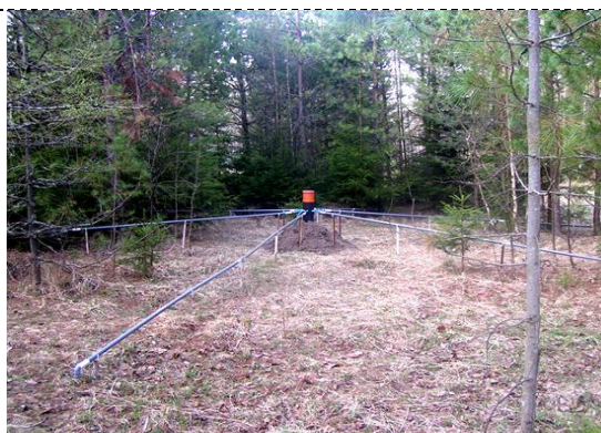
Figure 2. Appearance of MB-03 microbarometer with a system of wind-suppressing filters at the measuring platform
