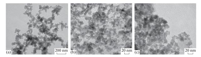
**Fig. 1.** TEM images of boehmite particles obtained by hydrothermal treatment of a nanosized  $\gamma$ -Al<sub>2</sub>O<sub>3</sub> powder in a 1.5 wt % HCl solution (a) at 200°C for 2.5 h, (b) at 170°C for 12 h, and (c) at 150°C for 36 h.
