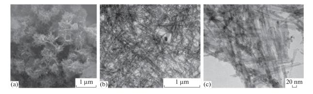
**Fig. 2.** (a) SEM and (b, c) TEM images of boehmite particles obtained by hydrothermal treatment of a nanosized  $\gamma$ -Al<sub>2</sub>O<sub>3</sub> powder in a 1.5 wt % HCl solution at 150°C for 96 h.
