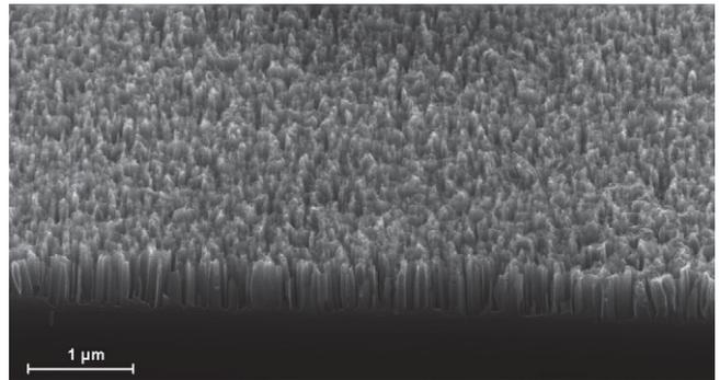
**Figure 1.** SEM image of a SiNW array recorded at a 70° tilt. The average nanowire height is 0.5 μm.
